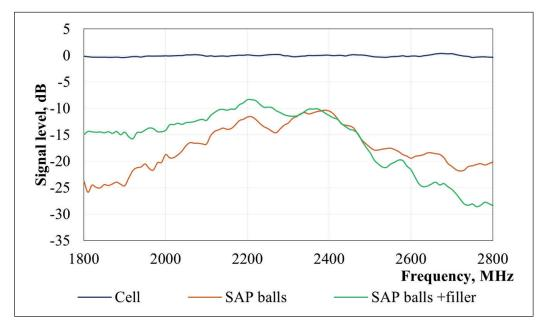
Fig. 4. Radio shielding with water-saturated superabsorbent polymers
