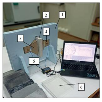
Fig. 1. Prototype of an installation for studying the radio shielding properties of materials in the microwave range: 1 -antenna holder (body), 2 -sample,
