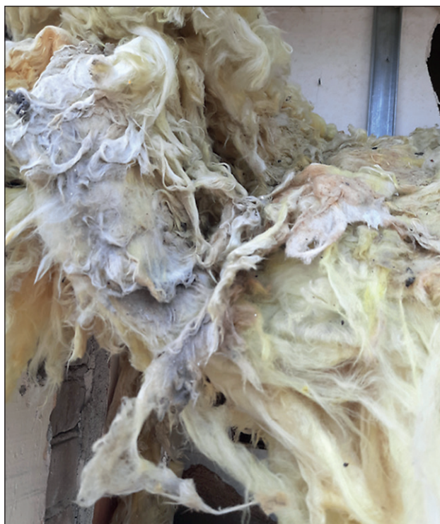
Fig. 12. A sample of mineral wool exposed to moisture The results of the experiment are shown in the figure 13
