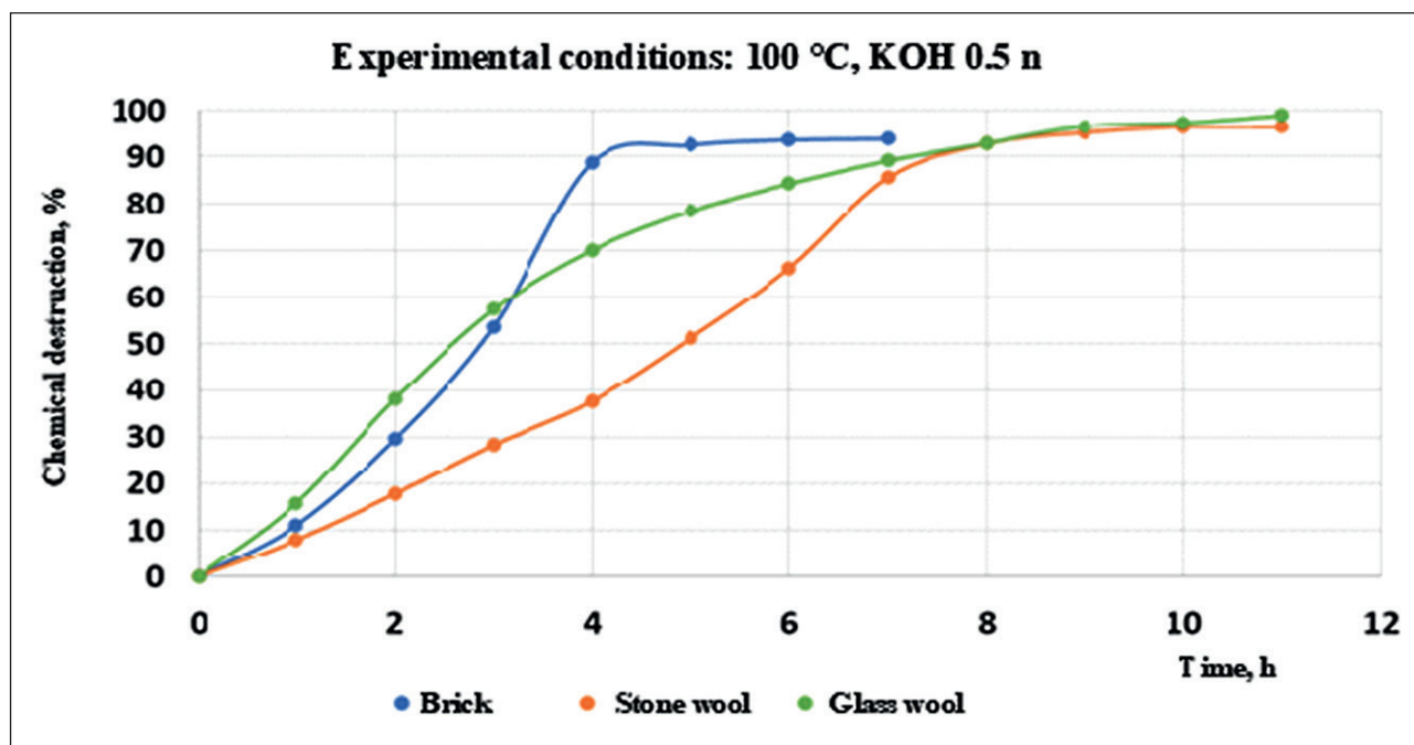
Fig. 6. Chemical degradation coefficient values for stone and glass wool in contact with 0.5 n potassium hydroxide at 100°C
