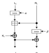
L<sub>i+1</sub> R<sub>i+1</sub> Figure. 7 Lightweight speck cipher
