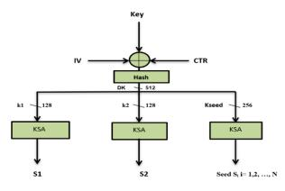
Figure. 5 Displays the proposed dynamic key generation and construction cryptographic primitives
