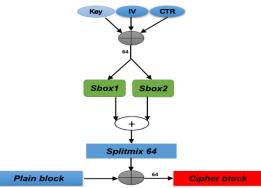
Figure. 6 Proposed lightweight encryption function
