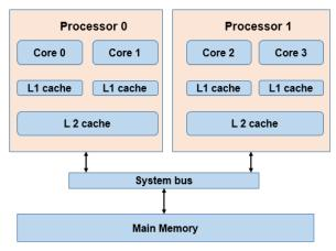
Figure. 2 Architecture of multi-core processor
