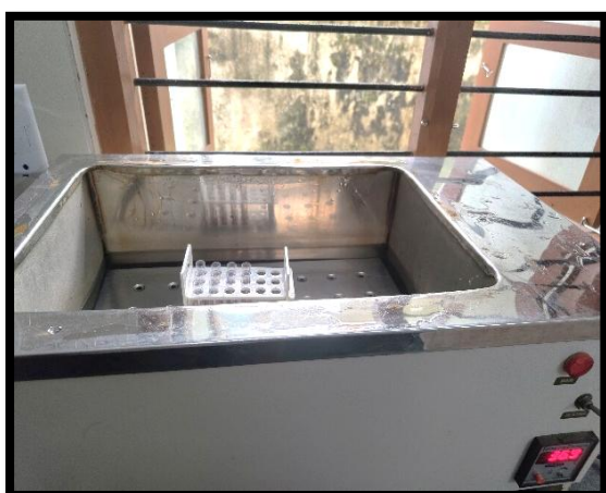
Figure 7 Incubating blood samples in water bath at 37°C
