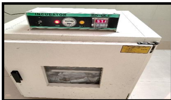
Figure 4 Drying the solutions in hot air oven at 57°C
