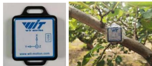
Fig. 5 – BWT61CL six-axis Bluetooth acceleration sensor
