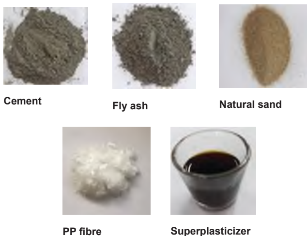
Fig. 3. Materials used for mixing concrete.
