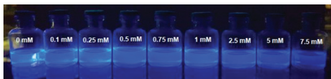
Fig. 4. Fluorescence quenching of DFDP in \text{CHCl}_3 (1 \mu\text{M} ) upon addition of mesotrione (0-7.5 mM).
