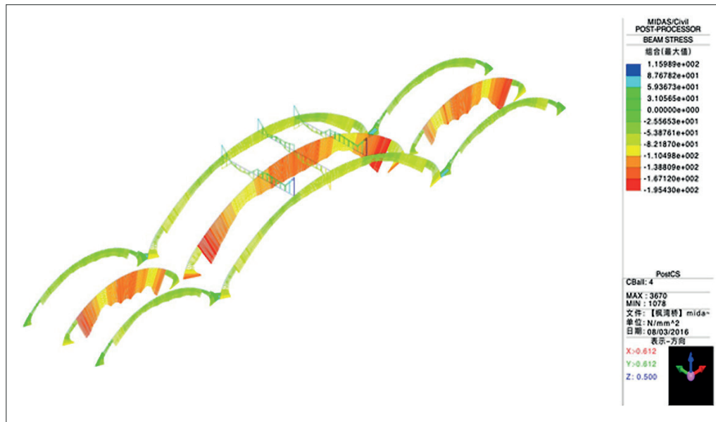
Fig. 6. The most unfavourable combination of action stress diagram
