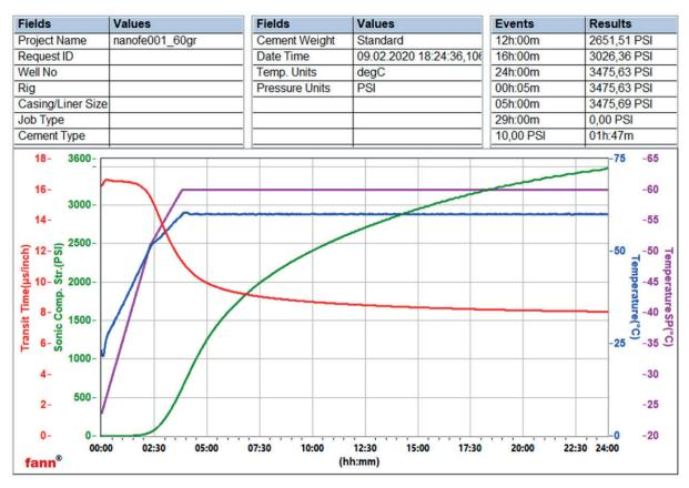
Fig. 6. Change in compressive strength of Portland cement stone with 0.01% nano iron powder at 60°C
