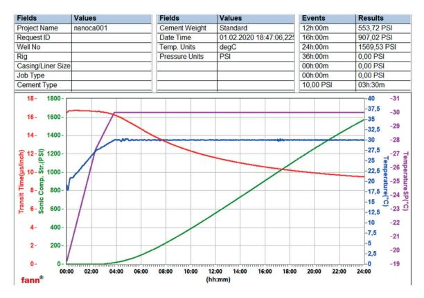
Fig. 2. Change in compressive strength of Portland cement stone with 0.01% calcium carbonate nanopowder at 30°C
