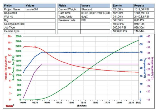
Fig. 3. Change in compressive strength of Portland cement stone with 0.01% nano iron powder at 30°C
