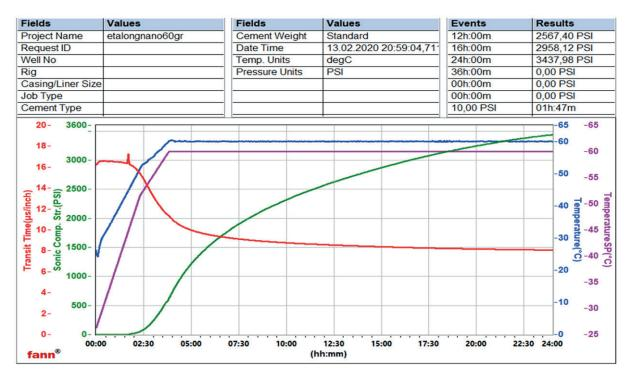
Fig. 4. Change in compressive strength of stone from additive-free Portland cement at 60°C
