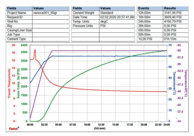
Fig. 5. Change in compressive strength of Portland cement stone with 0.01% calcium carbonate nanopowder at 60°C
