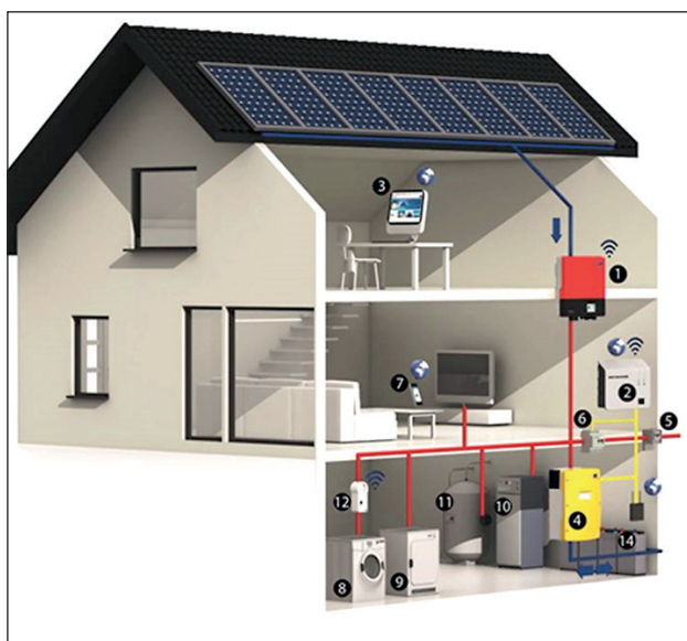
Fig. 2. Combined home heating / cooling system: 1 – Inverter; 2 – Controller; 3 – Remote control access; 4 – Battery; 5 – Electricity meter-detector; 6 – Compensator reactive power; 7 – Household electrical appliances; 8 – Washing machine; 9 – Dryer for clothes; 10 – Heat pump-vortex cooler; 11 – Electric boiler; 12 – Socket; 13 – Power grid; 14 – Router
