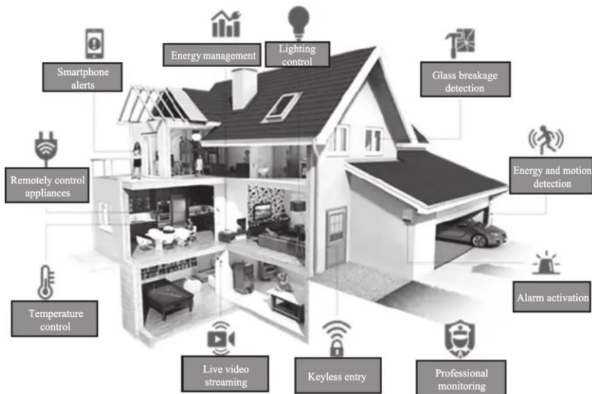
Figure 2. Schematic diagram of an IoT-enabled smart house depicting the employment of smart sensing devices in different utilities (IoT for smart house)
