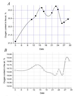
**Figure 6.** Graphs of changes in O<sub>2</sub> content (December 2019): a) calculated value, b) experimental value
