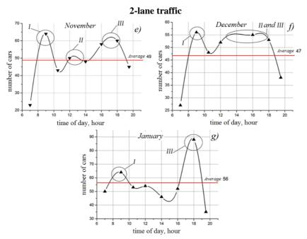
Figure 2. Graphs of changes in traffic intensity by the time of the day
