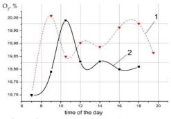
Figure 3. Combined graphs of changes in the number of cars and  $O_2$  content in the air during the day for 2-lane traffic roads (November 2019)1 – number of cars;  $2 - O_2$ content
