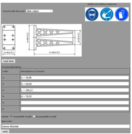
Figure 11. Conducting control with the application of slide caliper
