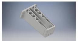
Figure 2. 3D CAD model of a car mirror holder
