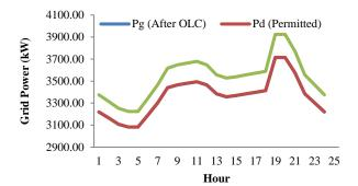
Fig. 1 Grid power drawn by MG before and after OLC by ATLBO
