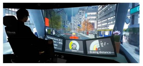
Figure 2. A virtual reality based SmartTram simulator. Tram operator's view in an autumn-evening lighting condition in an urban city environment. The rain and fallen leaves on the tramlines affect acceleration and stopping distance of the tram
