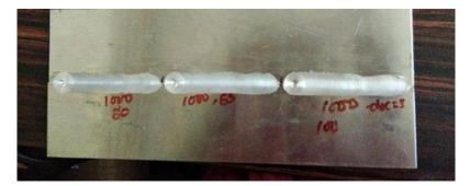
Figure 3: Resultant Al 6061 Alloys after Welding.
