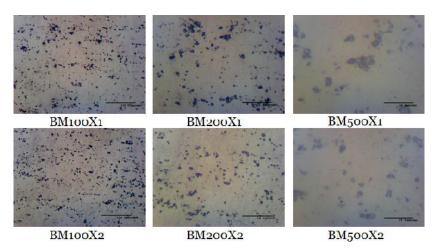
Figure 6: 6061 FSW S=1000 F = 100 Base Metal
