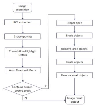
Fig. 8 - The image processing flow chart of damaged coated seeds
