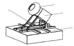
**Fig.1 - The overall structure of seed coating machine** 1- Coating pot; 2- Inclination adjusting device; 3- Rotary motor; 4- Vibrating table
