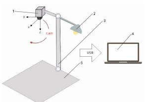
Fig. 2 - The mechanical vision experiment platform 1- USB camera; 2- Light source; 3- Bracket; 4- Image processing system; 5- Chassis
