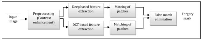
Figure 2. The blog diagram of the proposed novel method.
