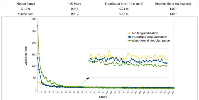
Figure 4. Effect of quaternion norm regularization on the validation loss. In the beginning of the training cumulative loss is significantly higher compared to the vanilla loss due to the chaotic estimations of the network. However, as the networks becomes more stable, constraint helps, optimization to find a slightly better minimum and faster convergence.
