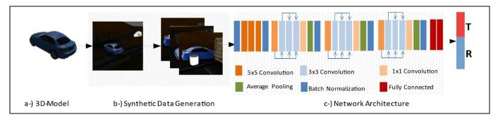
Figure 1. Direct estimation of camera poses with neural models using synthesized images. (a): Given a 3D model we generate random texture maps and distinct shapes and material properties. (b): We render images on dynamic and transparent backgrounds with varying illumination. Random 3D shapes and objects are placed between camera and the target object. (c): We train a custom densely connected custom neural architecture to directly estimate either camera or target object pose.
