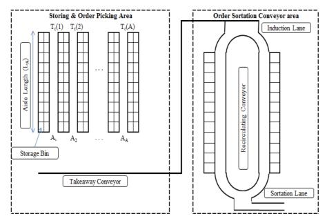
Figure 1: Top view of storing, order picking and sortation operation area
