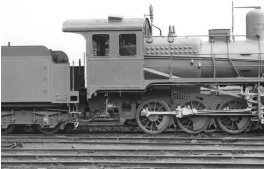
Figure 3. Shch class freight locomotive designed by Kharkiv Locomotive Plant (today, the Malyshev Factory). In total, about 2000 Sch class locomotives were manufactured by different plants in the 1900s – 1920s (Malyshev Plant, n. d.).
