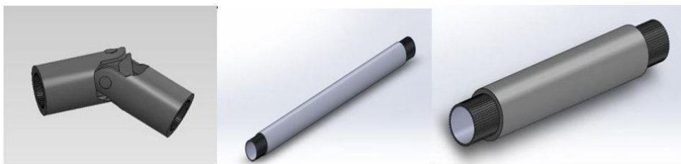
Figure 17: a) Universal joint(left) b) 325 mm steering column(right) c) 162 mm steering column(middle)
