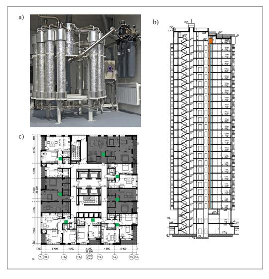
Fig. 7. MSA on the technical floor (a), section of a high-rise with nitrogen and air pipelines (b), floor layout with EGWMDS (c)
