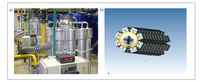
Fig. 4. Membrane separator of air ("a") and thermomagnetic separator of air ("b")
