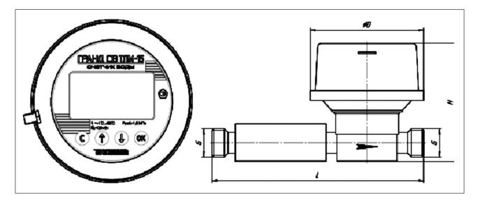
Fig. 5. Meters of cold and hot water with solenoid shut-off valves
