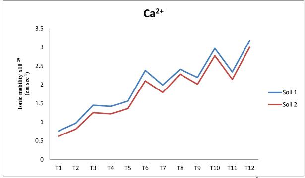
**Figure 6.** Comparing Ionic Mobility between the two Soils  $(Ca^{2+})$
