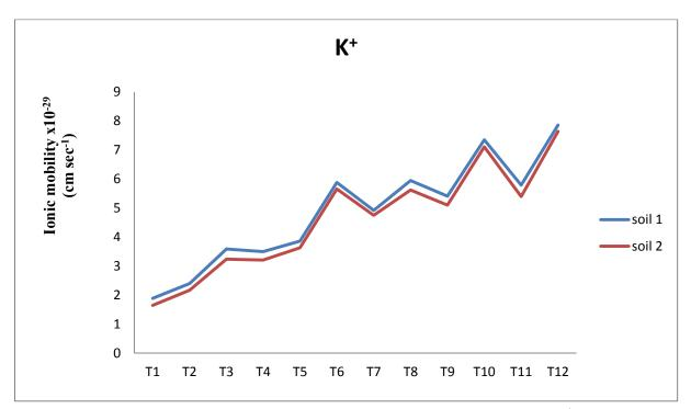
**Figure 9.** Comparing of Ionic Mobility between the two Soils  $(K^+)$
