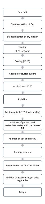
Figure 1: Manufacturing method for traditional doogh
