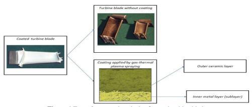
Figure 1. Tree of structural analysis of coated turbine blades
