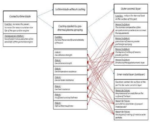
Figure 3. Failure analysis
