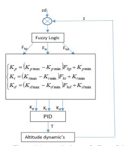
Figure. 4 A general scheme of a Fuzzy Gain-Scheduled PID (FuGSPID)
