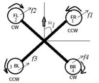
Figure. 1 A quadrotor configuration
