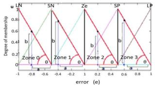
Figure. 7 Fuzzy sets with some triangle geometry.
