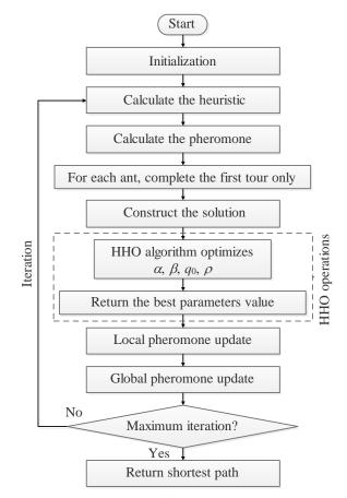
Figure. 4 Flowcharts of the HHO-ACS algorithm
