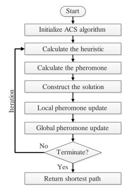
Figure. 2 Flowchart of the ACS algorithm
