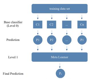
Figure. 4 The architecture of stacking
