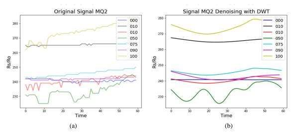
Figure. 7 Response signals: (a) Raw signal of MQ2 (b) Reconstructed signal of MQ2 after signal de-noising
