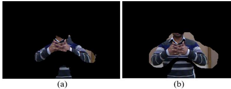
Figure. 3 Output image: (a) multilevel Otsu thresholding algorithm and (b) dilation disc operator
