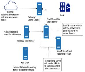
Fig. 1: Architecture of Malicious Servers Detection Schema for Preventing Client-Side Attacks
