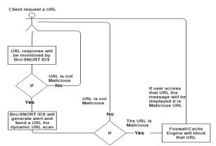
Fig. 2: Malicious Servers Detection Flow
