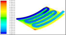
(c) 0.015 kilo-gram/sec fluid flow-rate Fig. 5: Temperature Contours of SFPC and SCPC for Changzhou City
