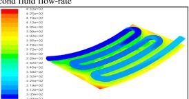
(c) 0.015 kilo-gram/second fluid flow-rate Fig. 4: Temperature Contours of SFPC and SCPC for Beijing City
