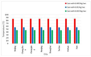
Fig. 3: Depart temperatures of functioning fluid regarding SCPC with eight unlike cities of China and varying flow-rates
