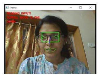
Fig 5.9 Operating cursor control system by a user wearing glasses
