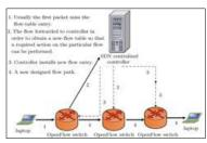
Fig. 12. Basic flow of works in SDN [33].
