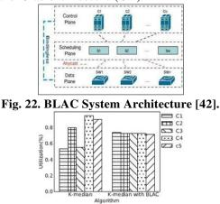
Fig. 23 Comparison between K-Median and Kmedian with BLAC for controller utilization [42].
