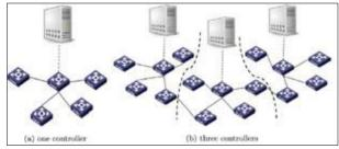
Fig. 10. Example of controller placement in star topologies with switch clustering [30].
