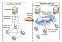
Fig. 9. Controller placement problem in the Wide Area Network (WAN) [27].
