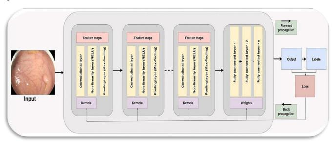
Fig.2 Convolutional Neural Network Architecture [6]
