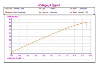
Figure 8: Multi Graph Report for Flexural Test 5 % Weight Fraction.
