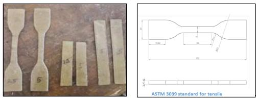
Figure 4: Testing Specimens
