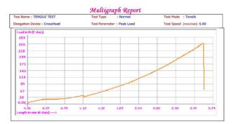
Figure 7:Multi-Graph Report of Tensile Test 5 % Weight Fraction.
