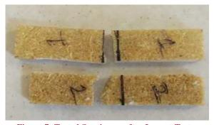
Figure 7: Tested Specimens after Impact Test.
