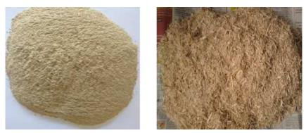
Figure 1: Sugarcane Bagasse Fibre.
