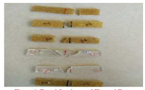
**Figure 6: Tested Specimens of Flexural Test**
