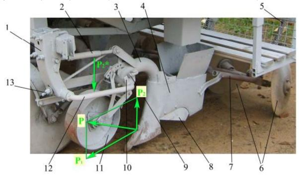
Fig. 2 – Coulter group of the KSU-4 clone potato planter (VIM) 1 – bracket attaching the coulter to the planter frame; 2 – upper link of the suspension; 3 – coulter bracket; 4 – coulter; 5 – push-rod; 6 – burrow-closing discs; 7 – disc mounting frame; 8 – blade; 9 – stop's adjusting bolt; 10 – stop; 11 – gauge wheel; 12 – lower suspension; 13 – Panhard rod
