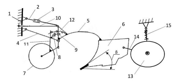
Fig. 4. – Coulter group of potato planters with automatic stabilization of planting depth
