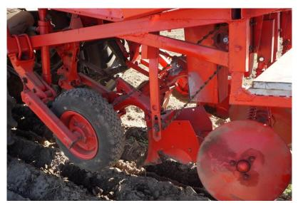
Fig. 5 - Experimental coulter group on VIM clone landing machine
