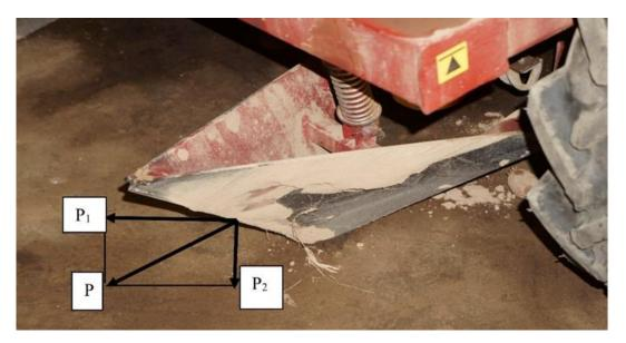
Fig. 1 – Coulter with a blunt angle of soil entry of L-202 potato planter  $P_1$  – is the tractor pulling force;  $P_2$  – is the force of the planter weight; P – is the resulting force
