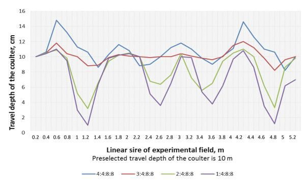
Fig. 8 – The effect of the coulter suspension ratio AB CD BC AD to the uniformity of the coulter travel when passing rough spots
