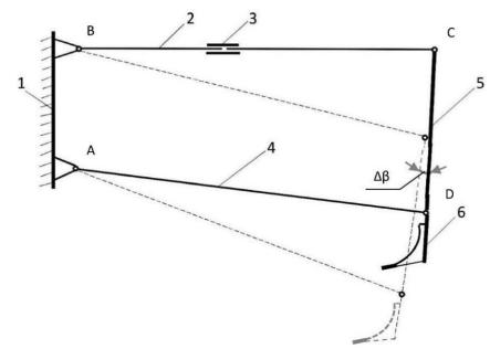
**Fig. 3 – Schematic diagram of the coulter individual floating suspension operation** 1 – planters to frame; 2 – longitudinal upper rods; 3 – telescopic coupling; 4 – longitudinal bottom rods; 5 – coulter body; 6 – coulter
