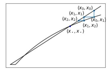
Figure 6. Plot of the curve y = f(x) - h, plot of the line y = x, and visualization of the evolution of the sequence  $x_n$  in the case h = 0.06.
