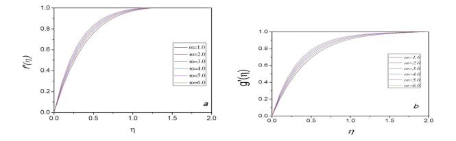
Figure 6. Plot of different velocity profile with respect to  $\eta$  on modification of  $\omega$
