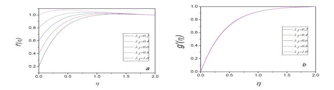
Figure 4. Plot of different velocity profile with respect to  $\eta$  on modification of  $\lambda_1$  fixed  $\lambda_2 = 0.0$
