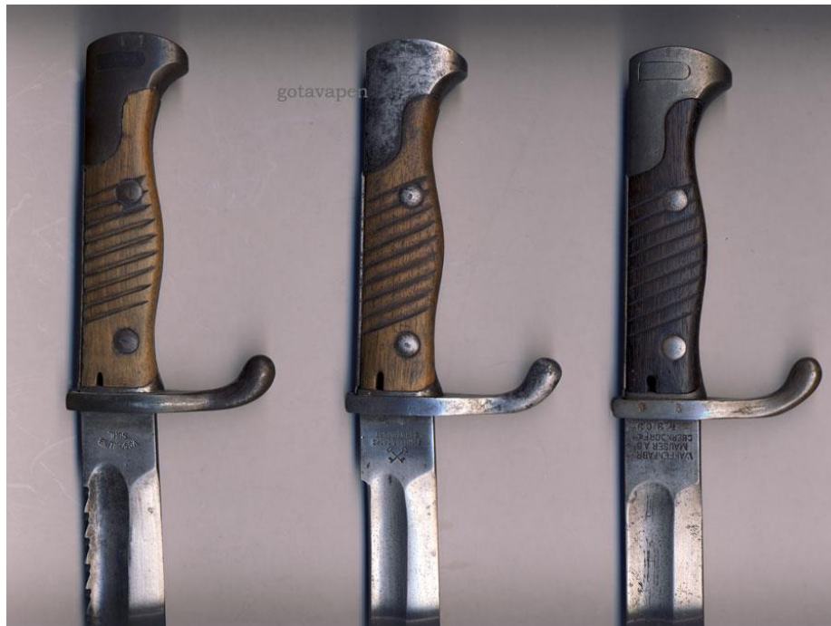
Figure 4. SG 98/05 bayonet with a saw (m.S. – mit Säge) with a ground-off saw (abg. – sägeabgeschliffen, which means “saw removed”) and without a saw (o.S. – ohne Säge) (Gotavapen, n. d.).
