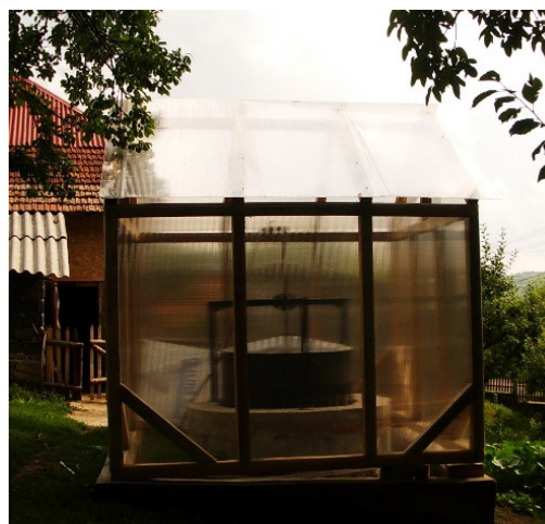
Fig. 3. Biogas unit prototype, digestion chamber of 4m 3 , in operation in Boteni, Arges county since 2010
