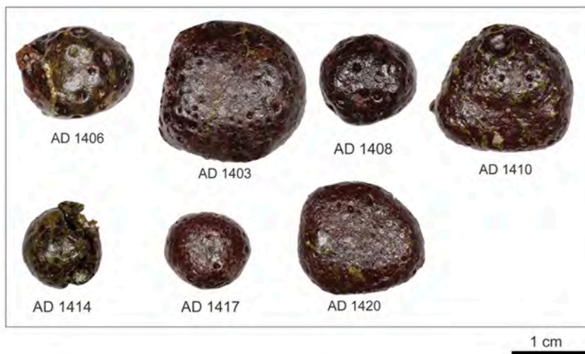
Fig. 11. Orheiul Vechi. Samples with MLT matrix type, samples after refiring at 1200°C. (Graphic preparation: Małgorzata Daszkiewicz/Hanna Baranowska).
