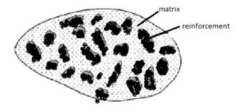
Fig. 1 Simplified scheme of a composite material [1].
