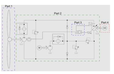
Figure 6. The subassemblies of the HST testing bench: Part 1 = wind turbine simulated with variable electric/ hydraulic motor; Part 2 = HST for low-power turbines; Part 3 = HST controller; Part 4 = synchronous generator.
