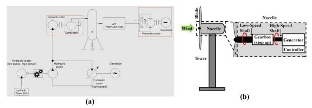
Figure 4. HST combined with energy pneumatic storage system (a), compared to a classical turbine (b).
