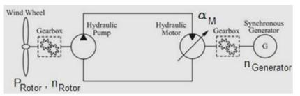
Figure 1. Fundamental principle of hydrostatic transmission (HST).
