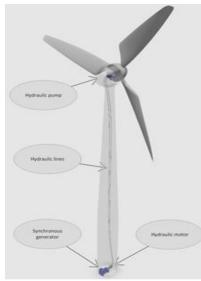
**Figure 5.** The main components of the wind turbine with HST
