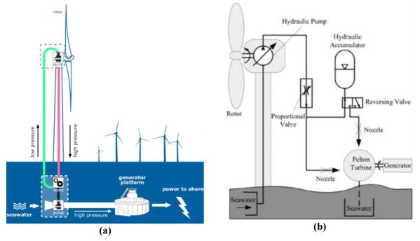
Figure 3. Offshore wind turbine with sea water: a) The principle works; b) Structure of the HST.
