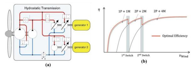
Figure 2. HST for a 1 MW turbine has been developed at IFAS: (a) Structure of the hydraulic scheme; (b) Diagram of system efficiency.
