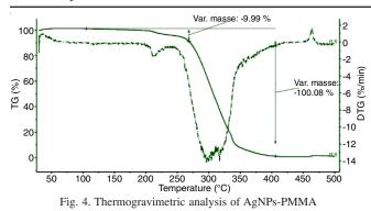
the flexible phase of polymer [23]. Fig. 4 also shows a thermal behaviour indicating a perfect dispersion of AgNPs within the chains of the polymethacrylate resin. Finally, in case of nanocomposite, the thermal degradation of material does not seem to be affected by the presence of silver nanoparticles.
