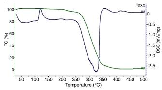
Fig. 5. Differential scanning calorimetry (DSC) of the mixture of AgNPs-PMMA
