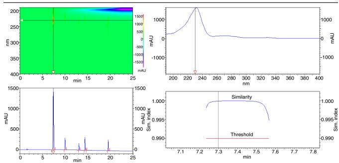
Fig. 5. Specificity chromatogram
