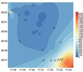
Fig. 4. Contour map of weighted arithmetic water quality index (WAWQI) of groundwater samples in study area
