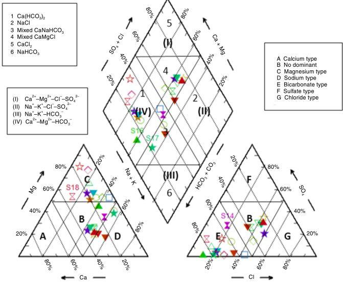
Fig. 9. Piper trilinear diagram of groundwater samples
