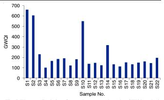
Fig. 5. Water quality index of groundwater samples using GWQI method
