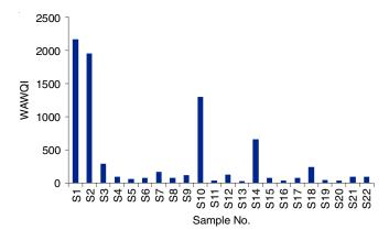
Fig. 3. Water quality index of groundwater samples using WAWQI method
