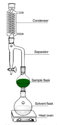
Fig. 1. System of the lemon peels essential oil extraction by the steam distillation method
