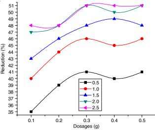
Fig. 2. Graphical representation on effect of *Tamarindus indica* L seed powder on the removal of chloride from drinking water without agitation
