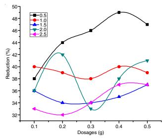
Fig. 1. Graphical representation on effect of *Tamarindus indica* L seed powder on the removal of chloride from drinking water with agitation
