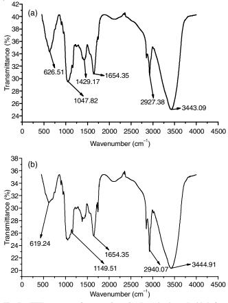
Fig. 7. FTIR spectrum of *Tamarindus indica* L seed polysaccharide before (a) and after (b) treatment
