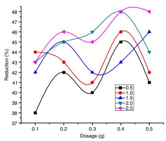
Fig. 3. Effect of *Tamarindus indica* L seed polysaccharide on the removal of chloride from drinking water without agitation
