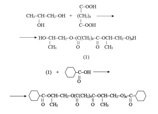
Synthesis of the polyester plasticizer was carried out by a two-stage method of condensation telomerization, since in this case oligoesters are more homogeneous in molecular weight and with a lower content of diesters compared to the one-stage method [34]. First, polycondensation of 1,2-propanediol and adipic acid was performed to obtain an oligoester with terminal hydroxyl groups, and then the resulting oligomer was esterified with cyclohexanecarboxylic acid.
